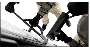
The MiniRam gives the MultiBreacher the required power to separate the door from the frame.
