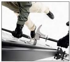
The MultiSledge can be used as a conventional sledge hammer in conjunction with the MultiPry for entry through outward opening doors.
