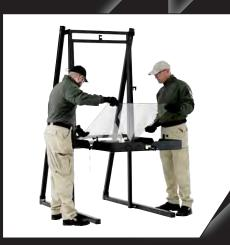
Different layers of glass or plastic sheets can be mounted to simulate various types of windows.
